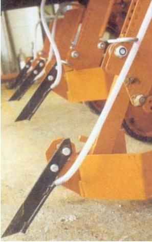
**Injector tines** Essentially tines cause soil disturbance and so must be thin in section but strong and durable to resist normal knocks and bumps and wear from abrasive soils. Our tines are machined and heat treated to give the required strength and wear resistance.
